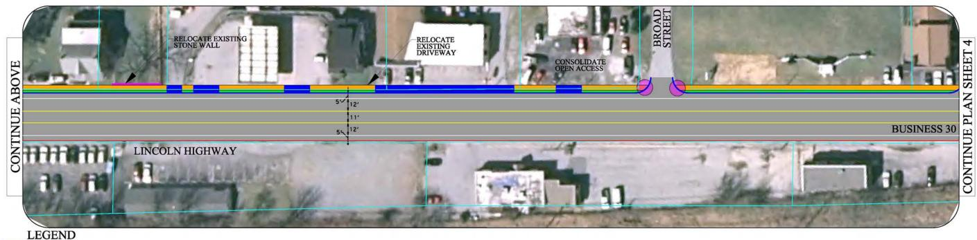
PROPOSED BUFFER AREA EXISTING PROPERTY LINE ROADWAY WITH PROPOSED PAVEMENT MARKINGS **EDGE OF ROAD** PROPOSED SIDEWALK PROPOSED CURB PROPOSED MEDIAN PROPOSED ADA RAMP UPGRADE
